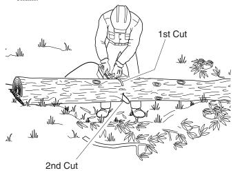
Figure 17 - Bucking Log When Log Is Supported
